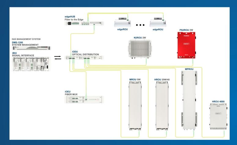
The SOLiD ALLIANCE 5G DAS efficiently delivers mobile network signals into commercial buildings, hotels, hospitals, airports, subways, stadiums, and any location where the outdoor network does not deliver the necessary in-building wireless coverage and capacity. SOLiD ALLIANCE remotes reduce the total cost of ownership with low power consumption, modularity to prevent rip-and-replace scenarios, and the highest bandwidth capability in the industry.
