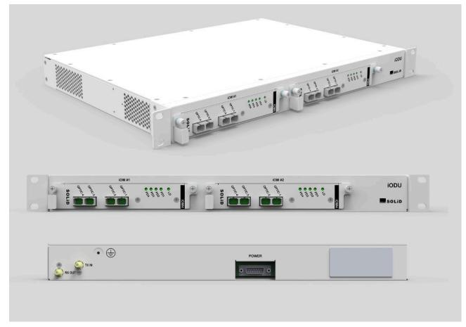
The integrated Optical Distribution Unit (iODU) receives downlink RF signals from the integrated BTS Interface Unit (iBIU), converts the RF signals to optical, then sends the signal to the remote optic units (ROUs) or to the Optic Expansion Unit (OEU or iOEU) via fiber optic cabling. This process is reversed for the uplink path.
