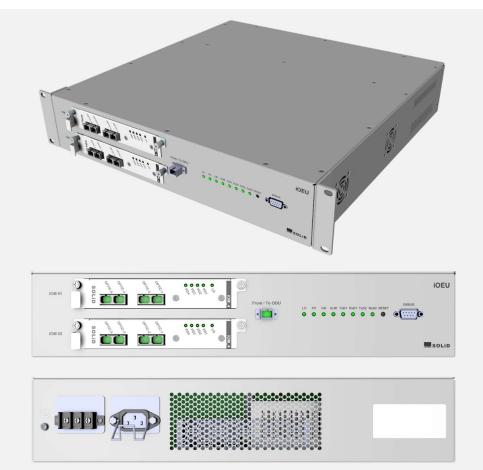
The integrated Optic Expansion Unit (iOEU) is an optional fiber MUX device designed to connect a DAS throughout multiple buildings or structures across a campus environment. The iOEU is typically located separately from the BTS Interface Unit (iBIU) headend and used primarily to drive multiple ROUs while limiting the amount of fiber required and increasing the optical link budget.
